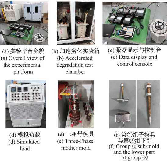
图 6 绕组绝缘多场景加速劣化模拟实验平台 Fig. 6 Multi-scenario accelerated degradation simulation experimental platform of winding insulation
