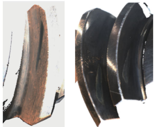
(b) 工业齿轮接触印痕: 镜像点云的彩色三维重建结果 (b) Industrial gear contact pattern: Color 3D reconstruction result of mirror point cloud
