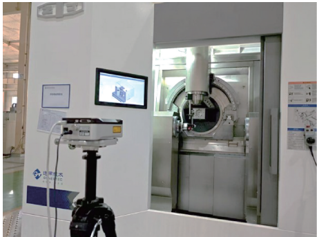
图 15 XR20 转角测量仪试验设置 Fig. 15 The XR20 angle measuring instrument experimental arrangement
