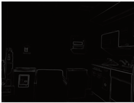
(b) Sobel算子边缘检测结果 (b) Edge detection results of Sobel operator
