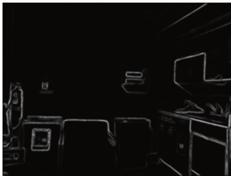
(c) 彩色图像边缘检测结果 (c) Edge detection results of color image
