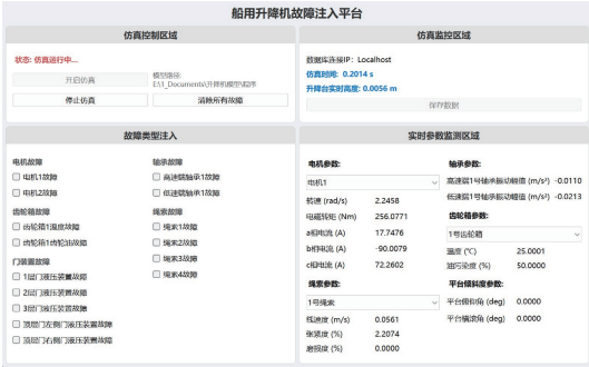
图 4 船用升降机故障注入平台界面 Fig. 4 Platform interface of the marine elevator fault injection
