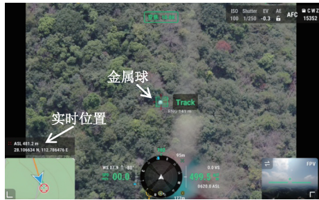
图 2 激光测距相机实时追踪金属球 Fig. 2 Real time tracking of metal sphere by laser ranging cameras
