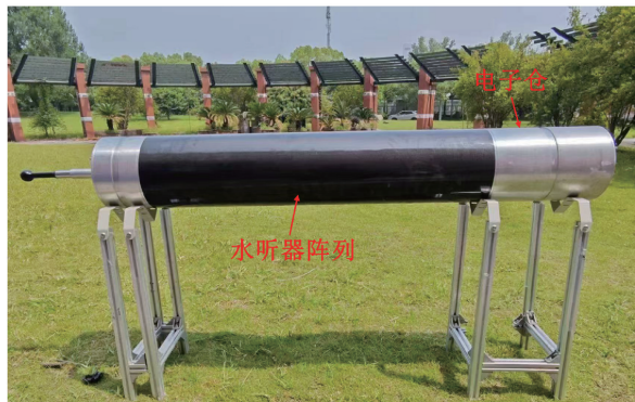
(b) 舷侧阵声纳系统 (b) Flank array sonar system
