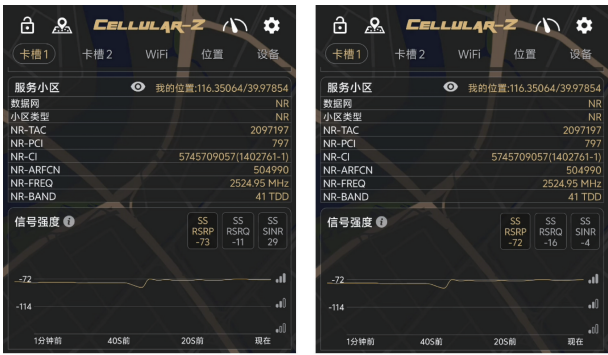
(a) 干扰发射前UE信号质量 (a) UE signal quality before interference transmission (b) 干扰发射后UE信号质量 (b) UE signal quality after interference transmission
