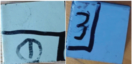
(b) 装配式钢结构防腐涂层金相试块 (b) Metallographic test blocks for anti-corrosion coatings of prefabricated steel structures
