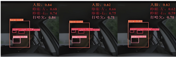
(b) 低照度环境检测效果可视化 (b) Visualization of low-illumination environment detection results
