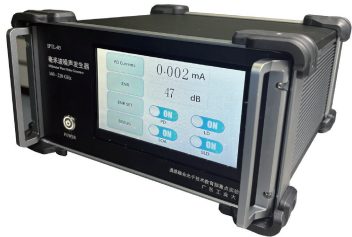
(b) 光子太赫兹噪声源实物 (b) Picture of photonic terahertz noise source
