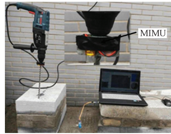
图 5 模拟钻进实验 Fig. 5 Simulated drilling experiment
