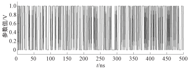
图 2 熵源节点输出信号的动态仿真结果 Fig. 2 Dynamic simulation results of the entropy source output
