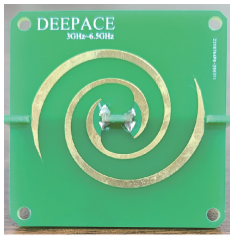
图 6 UWB-3 圆极化超宽带天线 Fig. 6 UWB-3 circularly polarized ultra-wideband antenna
