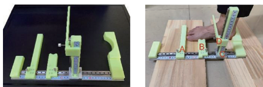
(a) AHIMS装置 (a) AHIMS device (b) 右足足弓指数测量 (b) Right foot arch index measurement
