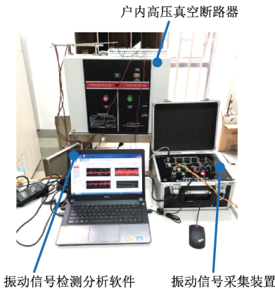
图 4 振动信号采集装置 Fig. 4 Field acquisition device for vibration signals
