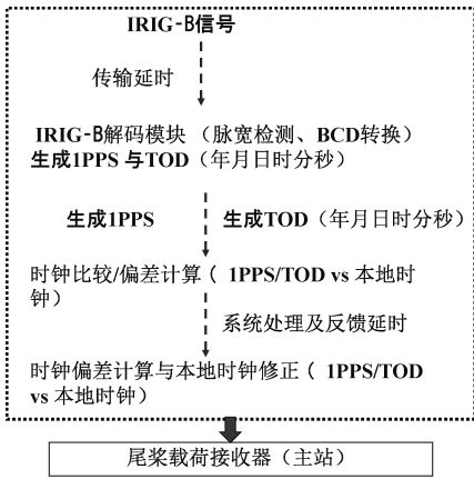
图2 基于IRIG-B信号时钟同步过程中的延时 Fig. 2 Based on the delay in the IRIG-B signal clock synchronization process
