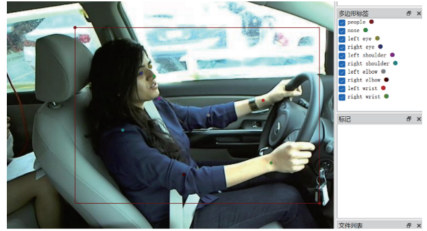
图 7 驾驶员关键点标注示意图 Fig. 7 Schematic diagram of driver key point annotation
